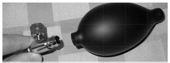
Inflation Bulb Leak Repair - Pull rubber bulb off the valve stem. Use a sharp pin to pry out the rubber check valve and wash it with dish detergent and hot water while squeezing and rolling it between your fingers to clean any fuzz from inside the valve. Do this over a bowl to prevent dropping it down the drain! Shake it dry then press it back into the valve stem. Press the bulb back on the valve stem. Done.
